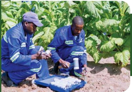
SAP technical officer collecting soil samples in a tobacco field using a soil probe and rubber mallet. The samples are stored in labeled containers for lab analysis to assess soil nutrients, pH, and moisture, aiding in precision agriculture and sustainable tobacco production.
