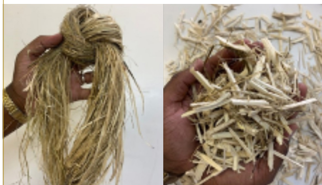
Fig 1.13 (a): Small-scale industrial hemp decorticator (b) Industrial hemp that has been decorticated and separated into shorter hurd and longer bast fibers, respectively.
